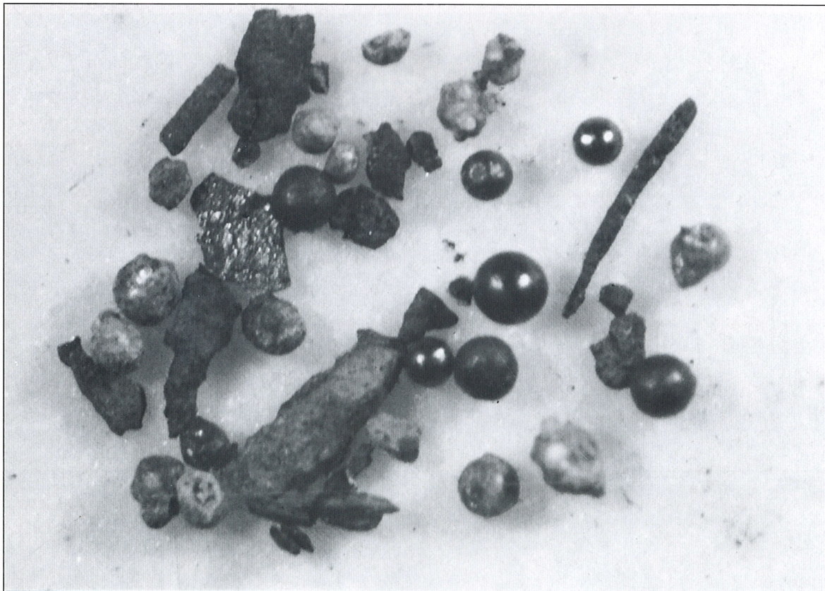
Figure 7. Heavy mineral assemblage of a strongly contaminated sample showing particles of tramp iron, magnetic spherules, and solder balls
