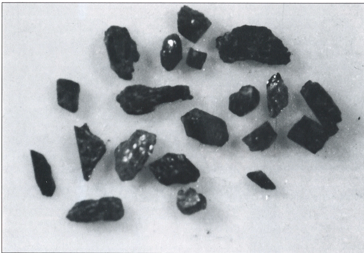
Figure 6. Heavy mineral assemblage in an uncontaminated sample showing ore minerals of cassiterite (tin) and wolframite (tungsten)
